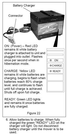
**NOTE:** Depending on extent of discharge and battery condition, allow approximately 16 hours for a complete recharge before additional use.
