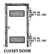
5. The following illustrations show minimum clearance dimensions for proper operation in a recess or closet installation.
