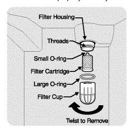
Order new filter cartridges through the dealer where you bought the refrigerator, or contact the *Sears PartsDirect at* 1-800-366-PART. It might be good to order some filter cartridges when you first install your refrigerator. Be sure to ask for the *Kenmore* replacement cartridge 46 9910.
