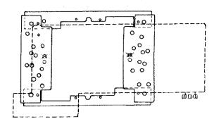
2. Mount the sander base to the end stiffener/channel support. Use two 5/16-18 x 2-1/2" hex head screws, flat washers, (4) external lockwashers, and (2) hex nuts.
