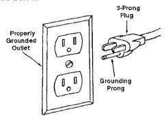
This power tool is equipped with a 3-conductor cord and grounding type plug listed by Underwriters' Laboratories. The ground conductor has a green jacket and is attached to the motor at one end and to the ground prong in the attachment plug at the other end. If repair or replacement of the electric cord or plug is necessary, do not connect the equipment grounding conductor to a live terminal.
