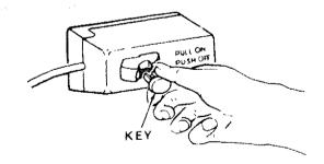
2. To turn machine on, insert finger under switch lever and pull end of switch out.
