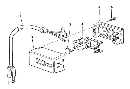
Figure 4 - On/Off Power Outlet 60382
