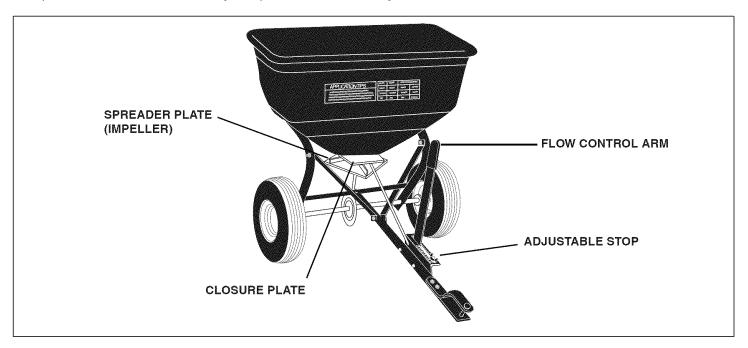
FLOW CONTROL ARM - Opens and closes the closure plate in the bottom of the hopper.
