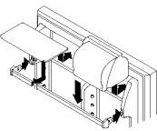
Adjust the utility compartment by lifting the front slightly and sliding it to the desired position. Lower the front to lock it into place.
