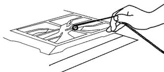
5. Push in and turn the burner knob to LITE/HI for the burner closest to the lit match. The burner will light immediately. When burner is lit, turn knob to desired setting.
