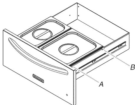
A. Position 1 pan support rail locator notch
