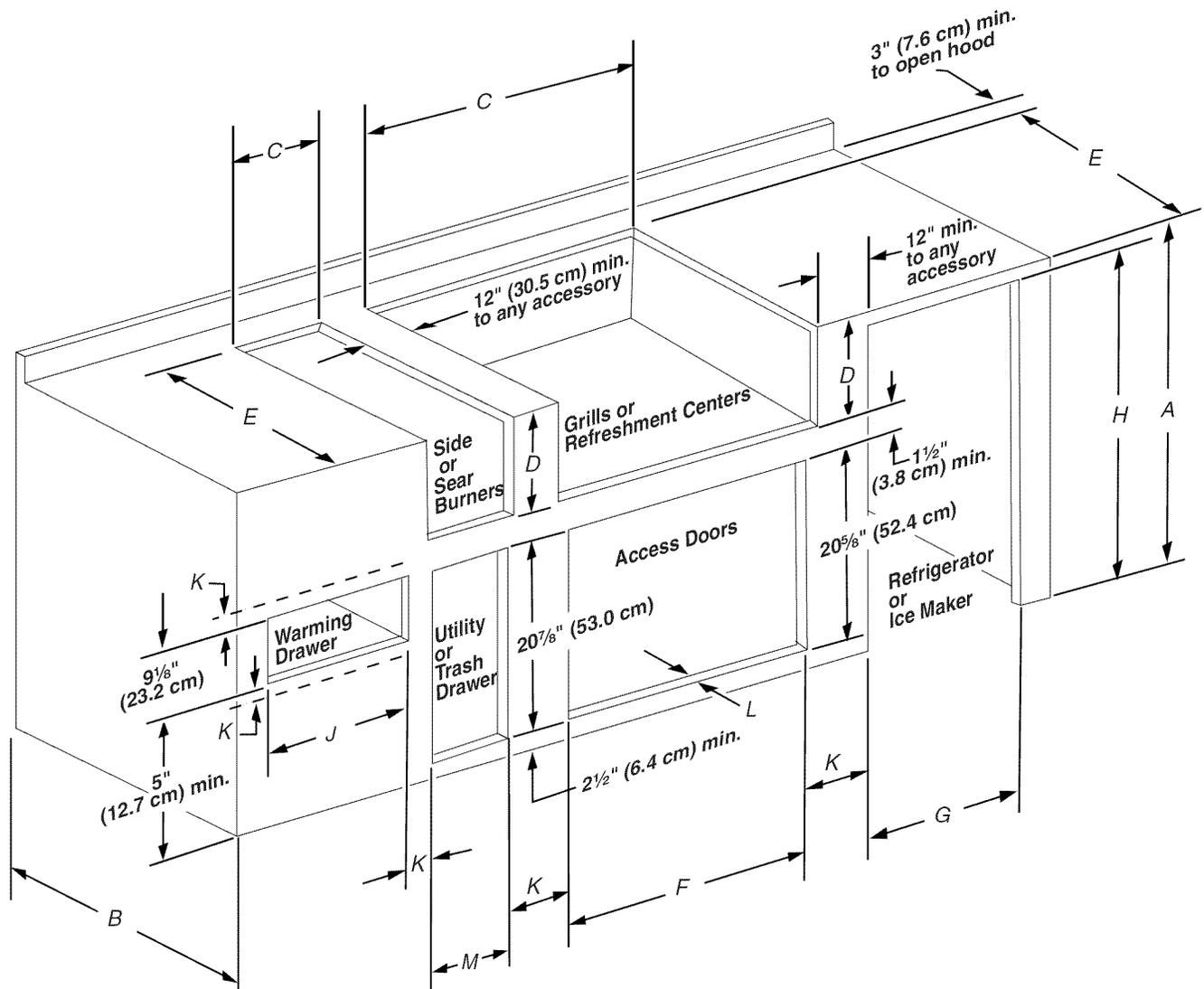
**Minimum Spacing Requirement Between Cutouts - Dimension K**
