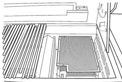
**NOTE:** View is shown with grates removed. Grates are to be in place when using the infrared sear burner.
