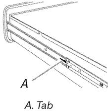
3. Press the tab down on the right side and lift tab up on the left side at the same time, then pull drawer out another inch to disengage latch.
