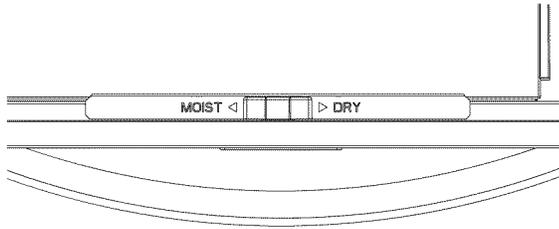
The Moist-Dry slide control allows you to open or close the vent slots in the door. The MOIST setting holds moisture in, while the DRY setting allows steam and moisture to escape from the drawer.
