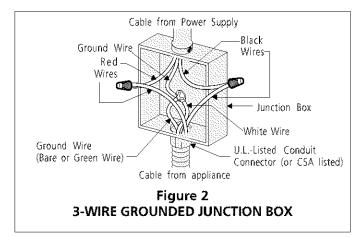
**AWARNING** Improper connection of aluminum house wiring to copper leads can result in a short circuit or fire. Use only connectors designed for joining copper to aluminum, and follow the manufacturer's recommended procedure closely.
