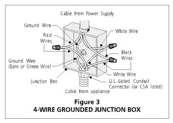
ACAUTION If connecting to a 4-wire electrical system, the appliance frame MUST NOT be connected to the neutral wire of the 4-wire electrical system.
