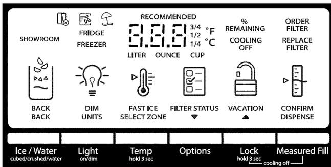
**IMPORTANT:** The display screen on the dispenser control panel will turn off automatically and enter “sleep” mode when the control buttons and dispenser paddles have not been used for 2 minutes or more. Press any control button to reactivate the display screen. The home screen will appear as shown.
