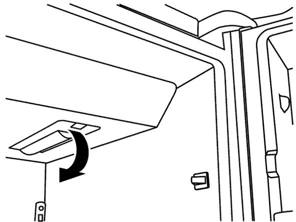
4. Align the arrow on the water filter label with the cutout notch in the filter housing and insert the filter into the housing.
