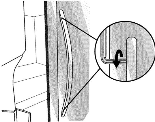
5. Using a clockwise motion tighten the setscrew just until it begins to contact the shoulder screw. Do not fully tighten.
