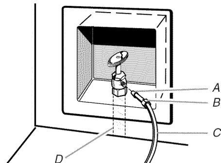
A. Sleeve      C. Copper tubing (to refrigerator)
