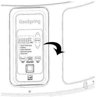
The bottom mounting screw can now be removed to access rear cover and wiring connections.
