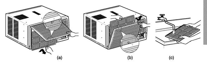
**CAUTION:** DO NOT operate the air conditioner without a filter because dirt and lint will clog it and reduce performance.
