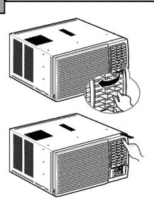
The direction of air can be controlled wherever you want to cool by adjusting the horizontal louver and the vertical louver.
