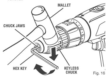
Open chuck jaws and remove hex key. Remove the chuck screw by turning it in a clockwise direction.
