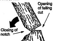
NOTE: Before felling cut is complete, use wedges to open the cut when necessary to control the direction of fall. To avoid kickback and chain damage, use wood or plastic wedges, but never steel or iron wedges.
