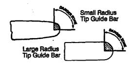
Low Kickback Chain has met kickback performance requirements when tested on the representative sample of these chain saws specified in ANSI B175.1.
