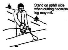
The chain saw operator should keep on the uphill side of the terrain as the tree is likely to roll or slide downhill after it is felled.
