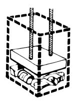
The compacting ram does not go to the drawer bottom. You will not see compacting of the first few loadings.
