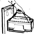
Remove bag carrier handles from side retainers and hold.
