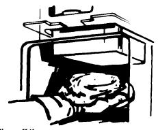
Wipe off the ram cover WARNING: To avoid personal injury from broken glass on the ram cover, wear rubber gloves.
