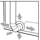
right, or straight out the back of the dryer. Space requirements are listed in your Installation Instructions.
