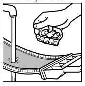
detergent; scrub lint screen with the brush to remove residue buildup.
