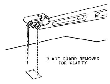
4. Locate the blade guard and carefully install it onto the saw as shown.
