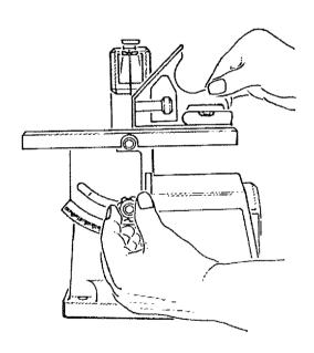
4. Loosen the screw holding the bevel scale pointer and adjust to 0°. Tighten screw.
