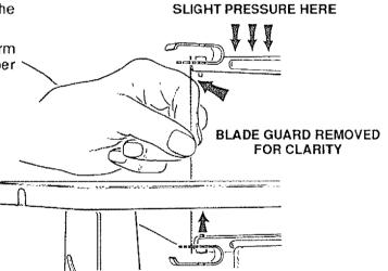
3. Look at the blade holders closely and notice the blade slots and pin recesses in the blade holder. The blade holder is made so you can position the blade for cutting from the front or one side of the saw.
