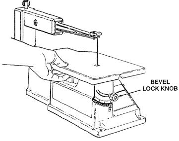
2. Use a small square to set the table at 90° to the blade. If there is too much space between the square and the blade, the table must be adjusted.
