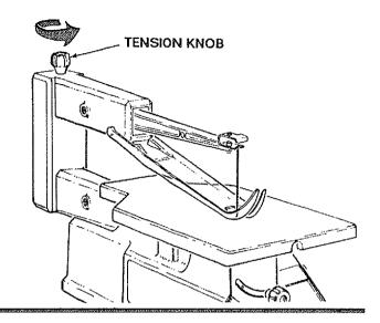
2. Remove blade by pulling forward on blade and then lifting the blade through the access hole in the table.
