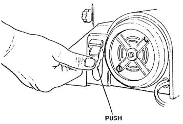
4. To lock switch in "OFF" position, hold switch IN with one hand, REMOVE key with other hand.
