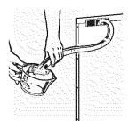
If the sink is 34" or higher from the floor, the excess water in Unicouple hoses cannot be drained directly into the sink. It will be necessary to drain excess water from hoses into a bowl or suitable container that is held outside and lower than the sink.
