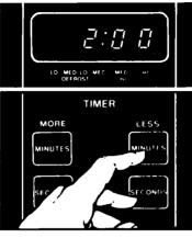
2. Press the MORE Minutes Pad until 1:00 shows on the Display. Continue to press or tap the pad until the Display shows the minutes of cooking time you want. To reduce the number of minutes on the Display, press or tap the LESS Minutes Pad until the proper number of minutes show on the Display.
