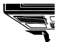
2. To remove grease filters, slide each filter to the side. Pull filters downward and push to the other side. The filter will drop out.
