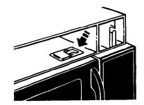
4. Remove bulb holder mounting screw.
