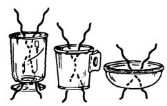
**Microwaves** pass through most glass, paper, and plastics without heating them so food absorbs the energy. Microwaves bounce off metal pans so food does not absorb the energy.
