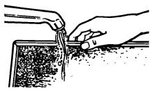
3. Soak grease filters in hot water and a mild detergent. Scrub and swish to remove embedded dirt and grease.
