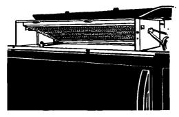
8. Slide a new charcoal filter into place. The filter should rest at the angle shown.
