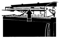
7. Lift the back of the charcoal filter. Slide the filter straight out.
