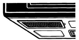
**11. Do not operate** the hood without the filters in place.
