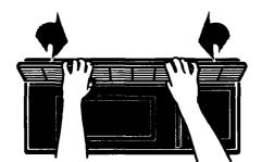
Slide the bottom of the vent cover into place. Push the top until it snaps into place. Replace the mounting screws. **10. Turn** the power back on at the main power supply.
