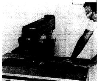
Fig. 108 - Hand and Body Position for Making an In-Rip Cut
