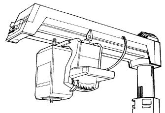
Fig. 111 - Arbor Shaft Position When Using Accessory Shaft
