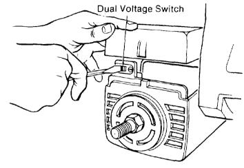
Fig. 135 - Dual Voltage Switch
