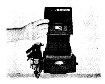
Fig. 27 - Miter Lock - Locked
