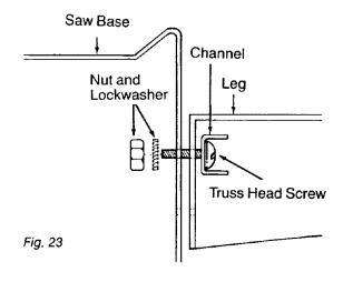
5. Position the front channel piece inside the legset. (Figure 23) Fasten the channel piece, leg, and saw together with two truss head bolts on each side. Put a lockwasher and hex nut on each bolt. The threaded section of the bolt should point towards the arm assembly.
