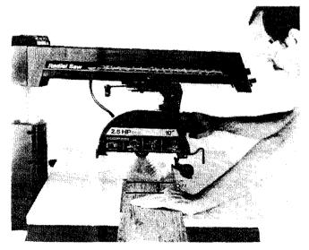
Fig. 97 - Hand Placement for Crosscuts
