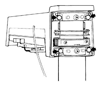
Fig. 127 - Location of Hex Head Tapping Screws
