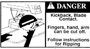
Fig. 3 Blade Contact Safety Sign
