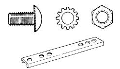
Fig. 22 - Bolt, External Lockwasher, Hex Nut, U-Channel
