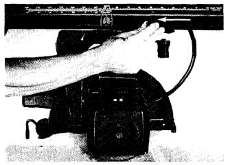
Fig. 32 - Rip Lock - Unlocked
