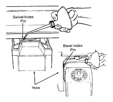
Fig. 122 - Swivel and Bevel Index Pins
