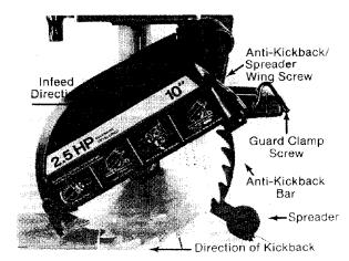
Fig. 106 - Blade Guard Position for Ripping
