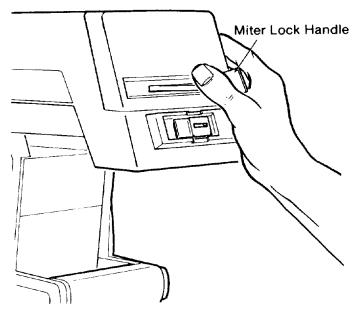
Fig. 131 - Miter Lock - Unlocked
