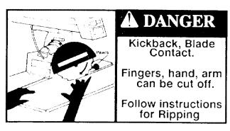
Fig. 101 - Kickback, Blade Contact Safety Sign
