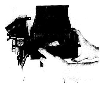
Fig. 29 - Bevel Lock - Locked
