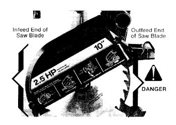
Fig. 104 - Infeed and Outfeed Ends of Saw Blade
