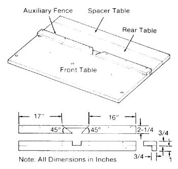
Fig. 117 - Auxiliary Fence for Edging
