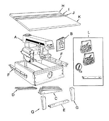
Fig. 10 - Parts for Model 113.197110 and 113.197150
