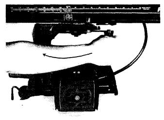
Fig. 30 - Swivel Lock - Unlocked
