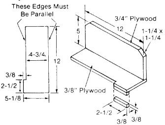
Fig. 115 - Push Block Dimensions
