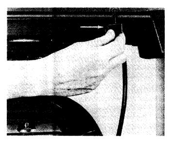
Fig. 92 - Locked Position for Rip Lock
