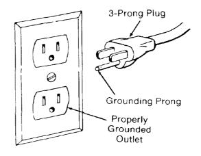
Fig. 83 - Plug for Less Than 150V
