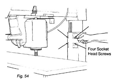
12. Use the top two screws to move the *radial* arm into line:
