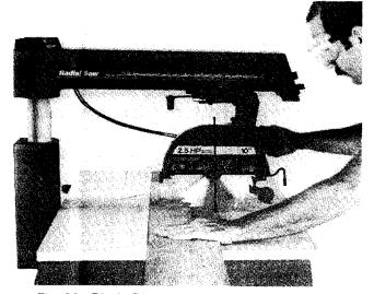
Fig. 90 - Blade Distance to Complete Crosscut
