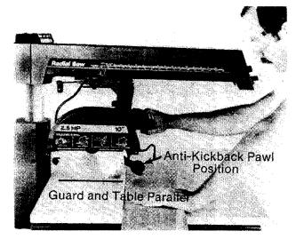
Fig. 94 - Crosscut Blade Guard and Body Position
