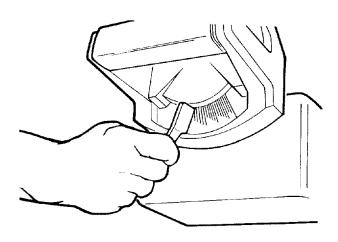
Fig. 124 - Bevel Lock - Locked
