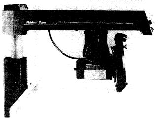
Fig. 100 - Out-Rip Saw Position (Infeed End)
