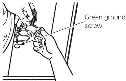
**⚠ WARNING:** IMPROPER CONNECTION OF ALUMINUM HOUSE WIRING TO THESE COPPER LEADS CAN RESULT IN A SERIOUS PROBLEM. USE ONLY CONNECTORS DESIGNED FOR JOINING COPPER TO ALUMINUM AND FOLLOW THE MANUFACTURER'S RECOMMENDED PROCEDURE CLOSELY.
