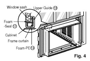
Pull each Frame curtain fully to each window sash track, and pull the bottom window sash down behind the Top retainer bar until it meets.
