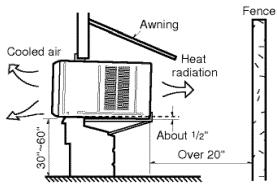
CAUTION: All side louvers of the cabinet must remain exposed to the outside of the structure.
