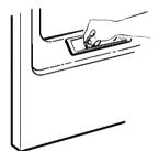
**The Exhaust Duct:** Inspect and clean the exhaust ducting at least once a year to prevent clogging. A partially clogged exhaust can lengthen the drying time.
