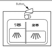
To open the wash cover, press the button and the cover will flip back.
