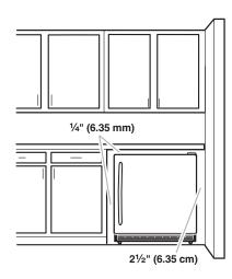
If your refrigerator is to be built-in, to ensure proper ventilation for your refrigerator, allow for 1/4" in. (6.35 mm) space on each side and at the top. When installing your refrigerator next to a fixed wall and the hinge side is next to the wall, leave 2-1/2" (6.35 cm) minimum to allow for the door to swing open. To open door wider, leave more space.
