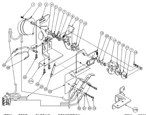
Item 27A: Models 76-1030-21 (115v-60Hz), 76-1030-22 (230v-60Hz) Item 27B: Models 76-1030-11 (115v-60Hz), 76-1030-12 (230v-60Hz)
