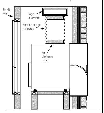
**2.** Secure the top duct to the unit by turning the four case top duct adjusting screws until they are tight. Use a field supplied clamp to lock the top duct to the case.
