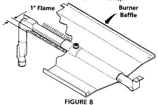
To determine if the oven burner flame is proper:
