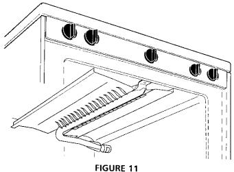
b. If adjustment to the air shutter is necessary, locate the broiler burner air shutter, loosen shutter set screw, and adjust to obtain optimum flame. This will normally be completely open for LP/Propane gas. If the flame is yellow in color, increase the air shutter opening size. If the flame is a distinct blue, but lifting away from the burner, reduce the air shutter opening size. Tighten the shutter set screw.
