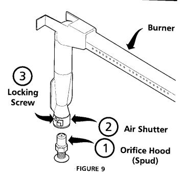
Retest the burner by repeating step "d" above. When the burner flame is a distinct blue color burning steady, the air shutter is adjusted correctly.
