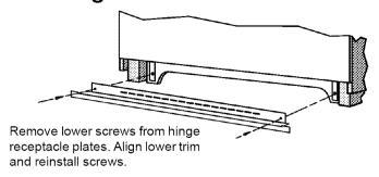
DO NOT INSTALL BOTTOM TRIM UNTIL UNIT IS ATTACHED TO THE CABINET.
