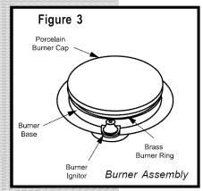
burner will ignite. Additionally, due to Vantage Flame™, the automatic reignition feature, the igniters will spark automatically if a flame should blow out or be severely distorted by a draft or by a ventilation system. Burner igniters must always be kept clean and dry to function properly. Dirty or wet igniters will result in constant sparking, even if there is a flame present. See **Figure 3**.
