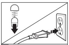
Make sure the Speed Control is in the "OFF" position by sliding it backward as far as possible. "OFF" will be visible on the speed control pad. Then plug the Hand Mixer into an electrical outlet.
