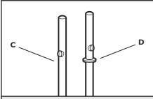
Paired accessories (beaters, optional dough hooks) include one accessory with a collar (D), and one without (C). Single accessories come with a collar (D) (liquid blending rod) or without (C) (whisk).
