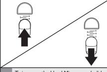
To increase the Hand Mixer speed, slide the Speed Control forward. To decrease the Hand Mixer speed, slide the Speed Control backward. See "Speed control guide" section.
