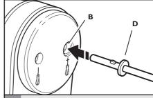
Insert the accessory shaft with the collar (D) into the larger opening (B) of the hand mixer. Align the flanges on the shaft with the slots in the opening. Push to lock into place.
