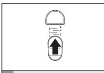
Start mixing at the lowest speed by sliding the Speed Control forward to the first position mark, which is Speed 1.
