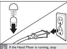
If the Hand Mixer is running, stop the Hand Mixer by sliding the Power switch to "OFF". Then unplug from the electrical outlet.
