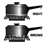
Never extend the flame beyond the outer edge of the utensil. A higher flame simply wastes heat and energy, and increases your risk of being burned by the flame.
