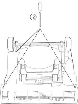
2. Remove 3 base plate screws using a Phillips® screwdriver. Lift base plate off base.
