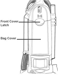
1. Release front cover latch by lifting up. Pivot bag cover away from cleaner and remove.
