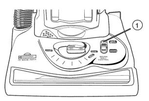
1. Move brush roll control lever to hard floor position.
