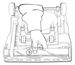
5. Insert right end into base. Make sure it is fully into position. Ensure belt is centered. **NOTE: The new belt will appear to be too large. This is normal.**
