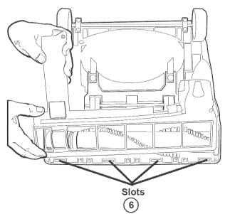
6. Replace base plate by first inserting all 4 front tabs into slots on base. Rotate down on cleaner and replace 3 screws.
