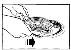
3. Hold the surface unit as level as possible with the terminal just started into the receptacle. Push the surface unit terminal into the receptacle.
