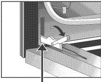
Lock engaged for door removal Figure 2
