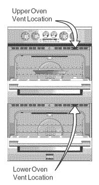
! CAUTION This model is equipped with a blower which runs in baking and self-cleaning mode to keep all internal components at a cool temperature. The blower may keep running even if the oven has been turned off, until the components have cooled down. In self-clean mode, the blower in both ovens will start when using one of the ovens.
