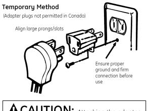
**ACAUTION:** Attaching the adapter ground terminal to the wall receptacle cover screw does not ground the appliance unless the cover screw is metal, and not insulated, and the wall receptacle is grounded through the house wiring. The customer should have the circuit checked by a qualified electrician to make sure the receptacle is properly grounded.
