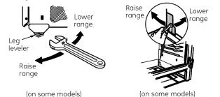
**B.** Check for levelness by placing a spirit level or a cup, partially filled with water, on one of the oven racks. If using a spirit level, take two readings—with the level placed diagonally first in one direction and then the other.
