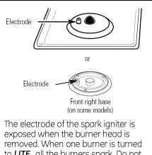
removed. When one burner is turned to **LITE**, all the burners spark. Do not attempt to disassemble or clean around any burner while another burner is on. An electric shock may result, which could cause you to knock over hot cookware. Installation Instructions
