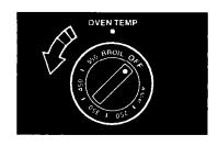
6. When broiling is done, turn the Oven Temperature Control Knob clockwise to OFF.
