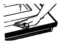
OVEN BOTTOM AND INSIDE SURFACE OF DOOR – Wash with warm, soapy water. Use a steel-wool pad or plastic scrubbing pad for heavily soiled areas. Wipe well with clean water.
