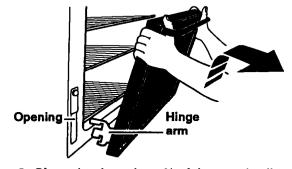
3. Close the door about 3/4 of the way (until it is 1/4 open). Grasp the door firmly on both sides and lift up and off the hinges.
