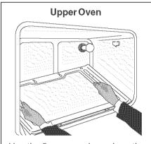
Use the finger openings along the outside edges of the oven bottom to remove the oven bottom.
