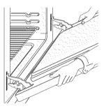
HINGE SLOT - Door removed from the oven Figure 2 - Single Oven Models
