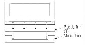
• Secure the bottom trim to the bottom of the oven using 3 screws provided.
