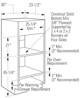
\* For existing cutouts, a maximum width of 28-1/2" is acceptable. If the opening is slightly wider, secure a furring strip on each side of the cutout for securing the oven.
