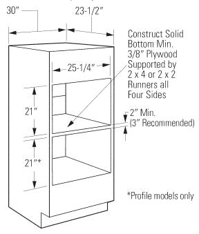
• If you are mounting an Under-the-Counter GE/Monogram oven over another, use the dimensions shown. The middle rail separating the two openings may need to be larger than the 2" minimum shown.
