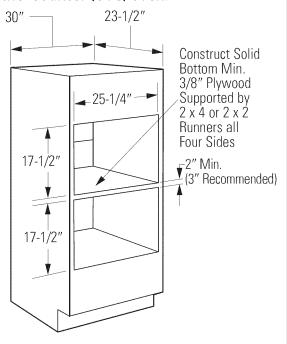
• If you are mounting an Under-the-Counter GE/Monogram oven over another, use the dimensions shown. The middle rail separating the two openings may need to be larger than the 2" minimum shown.
