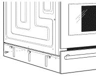
D Place the side supports into the tabs on the drawer and secure using the screws supplied and the screws removed in Step C.
