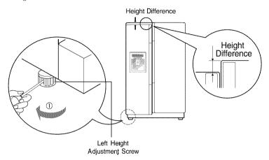
If the freezer compartment door is higher than the refrigerator compartment door Level the door by inserting flat ( - type) driver into the groove of the right height adjusting screw and rotating it clockwise  $\mathbb{O}$ .
