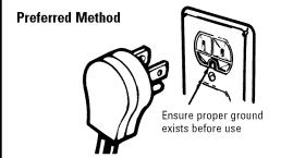
The power cord of this appliance is equipped with a 3-prong (grounding) plug which mates with a standard three-prong grounding wall receptacle to minimize the possibility of electric shock hazard from this appliance.
