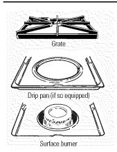
CAUTION: Do not operate the cooktop without all burner parts, drip pans (if so equipped) and grates in place.
