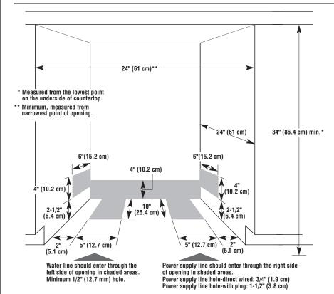
Drain hose should enter through cabinet in shaded areas. Drain hose size: 1-1/2" (3.8 cm)
