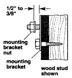
**5** ■ Space the mounting bracket nuts 1/2" to 3/8" away from mounting bracket.
