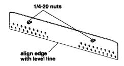
Align the lower edge of the mounting bracket assembly with the level line. Select and mark a hole location on each side of the bracket that is closest to the center of each stud.
