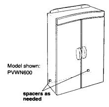
Check tops of doors for uniform vertical alignment. Wall irregularities may require shimming the back bottom corners of the cabinet away from wall to align the door tops.
