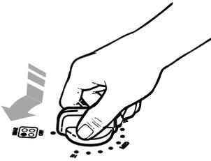
2. **After the burner lights**, turn the control knob to the desired setting.
