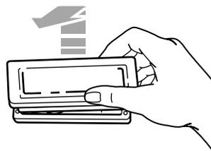
2. **Remove** glass light cover by grasping front edge of cover and pulling it away from side wall of oven.
