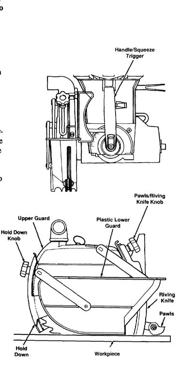
the pawls/riving knife knob. When lowered for crosscutting, it acts as a barrier to the leading edge of the blade.
