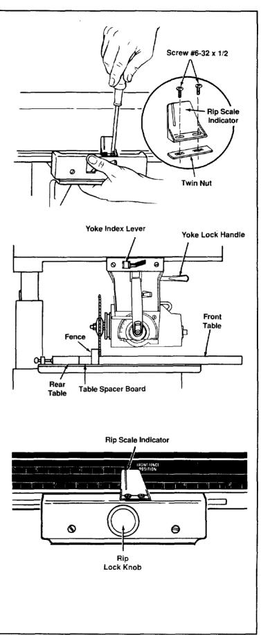
6. The blade "Out-Rip" scale indicator on left hand side of the radial arm is adjusted in essentially the same manner as blade "In-Rip" indicator, except position blade with 2 inches between fence and face of saw blade. The rip-scale indicator should be positioned to read 2 inches on upper portion of the blade "Out-Rip" scale.
