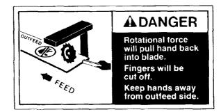
If you reach around the blade to the outfeed side when ripping, and try to hold down or pull the workpiece through to complete a cut, the rotational force of the blade will pull your hand back into the blade.
