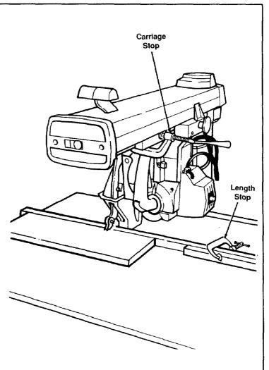
5. When making miter or bevel cuts, use extra force to hold workpiece down because it tends to move during these types of cuts.
