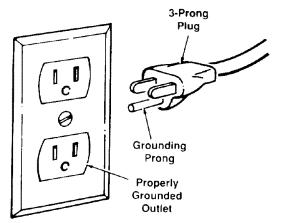
The power tool is equipped with a 3-conductor cord and grounding type plug listed by Underwriters' Laboratories. The ground conductor has a green jacket and is attached to the tool housing at one end and to the ground prong in the attachment plug at the other end.
