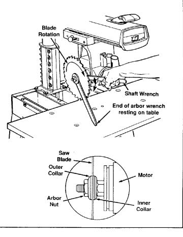
3. Lower arm until saw blade just clears the front table. Lock the yoke lock handle and bevel lock lever.
