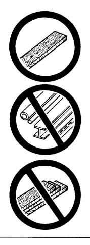
3. Rip only workpieces longer than the diameter of the blade. Do not rip workpieces that are shorter than the diameter of the blade being used.
