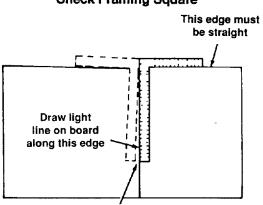
Should be no gap or overlap here when square is flipped over to dotted position.
