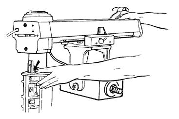
2. Loosen (2) 1/4 - 20 Gib socket cap screws on the left side at the rear of the column support slightly (1/2 turn).
