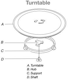
The turntable can rotate in either direction to help cook food more evenly. For best cooking results, do not operate the microwave oven without having the turntable in place. See "Assistance or Service" to reorder any of the parts.
