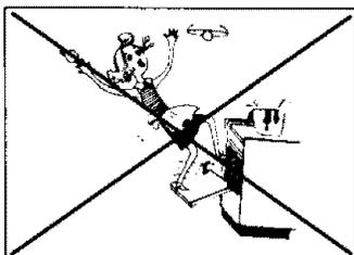
Do not touch a hot oven light bulb with a damp cloth as the bulb could break. Should the bulb break, disconnect power to the appliance before removing bulb to avoid electrical shock.
