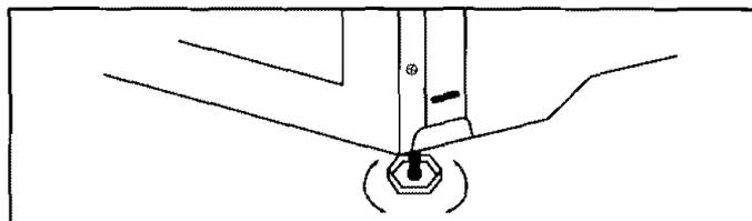
**WARNING:** To reduce the risk of accidental tipping of the range, it must be secured by an anti-tip device. To check if the device is installed properly, use a flashlight and look underneath the range to see that one of the rear leveling legs is engaged in the bracket slot.
