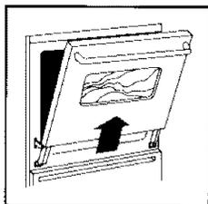
**To Replace Oven Door:** Grasp the door at each side, align the slots in the door with the hinge arms and slide the door down onto the hinge arms until it is completely seated on the hinges.
