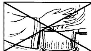
Always place oven racks in the desired positions while oven is cool. If a rack must be moved while hot, use a dry potholder and avoid touching hot element in oven.
