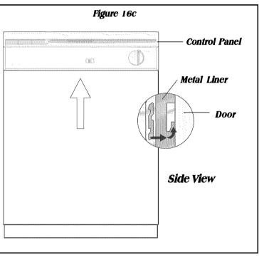
6. Unlatch door and open while supporting outer door on both sides at bottom to keep in place. Align screw holes and replace screws.
