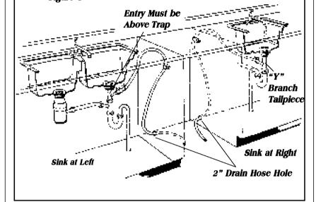
2. If you connect to a sink drain, entry will need to be above trap. A "Y" branch tailpiece and connector kit, not included, will make this method easier and includes all needed fittings and instructions. See Figure 5.
