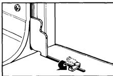
3. Rotate the Broil Stop clips over the door hinge slots and close the door to the Broil Stop position (open about 4 inches, 10.2 cm). The door will stay open by itself.
