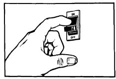
WARNING: To avoid possible shock hazard, turn off the electric power at the main power supply.
