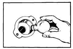
2. Remove the light bulb from its socket. Replace with a 40-watt appliance bulb. Turn the power back on at the main power supply.
