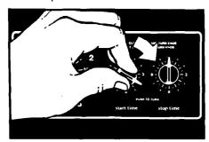
3. Push in and turn the Start Time Knob clockwise to the time you want baking to start.
