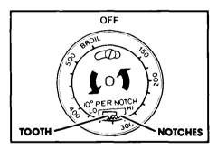
**3.** To lower the temperature, move the tooth a notch closer to LO. Each notch equals about 10°F (5°C).
