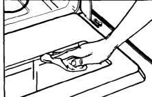
WINDOW – Keep clean with hot soapy water. Use a plastic scrubbing pad for stubborn spots. Rinse well. Do not use steel wool or abrasive cleansers.
