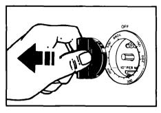
**1.** Pull the Oven Temperature Control Knob straight off.
