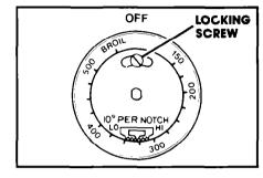
2. Loosen the locking screw. Note the position of the notches.
