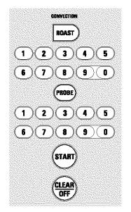
To change the oven temperature during the Convection Roast cycle, touch the **CONVECTION ROAST** pad and then touch the number pads to set the new desired temperature.
