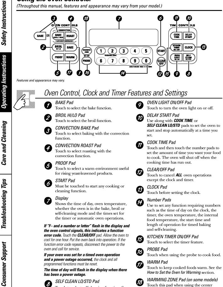
Touch to select self-cleaning function. See the Using the self-cleaning oven section.
